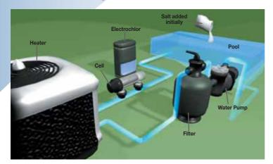
The Electrochlor is plumbed directly in-line with the pool equipment, typically after the heater. The power control unit is wired to the pool timer so it sanitizes the water when the pump is running.
